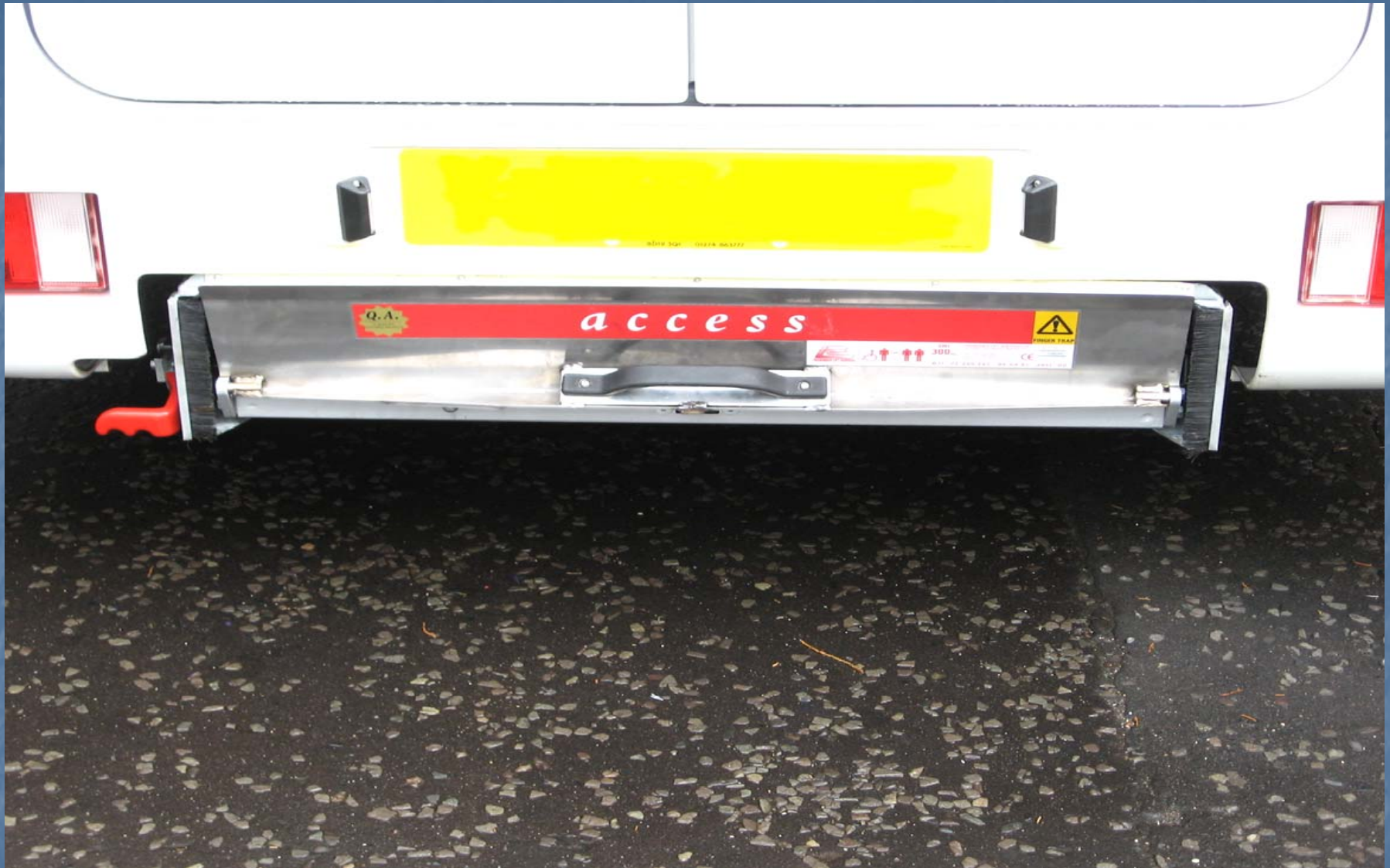
Access Lift is stowed away.
